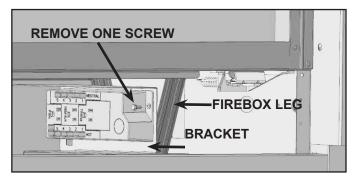
Figure 8.2 Junction Box Detail - JADE42IN-B, JADE42IL-B
