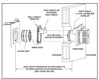
Figure 7.12 Venting Through the Wall
