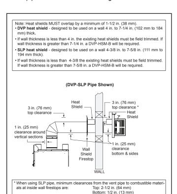
Figure 5.1 Horizontal Venting Clearances To Combustible
