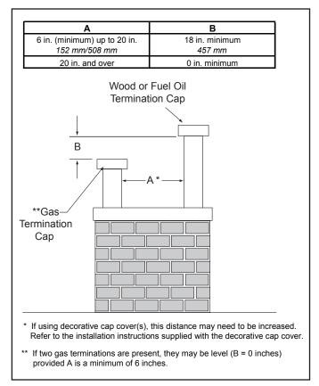
Figure 4.2 Staggered Termination Caps
