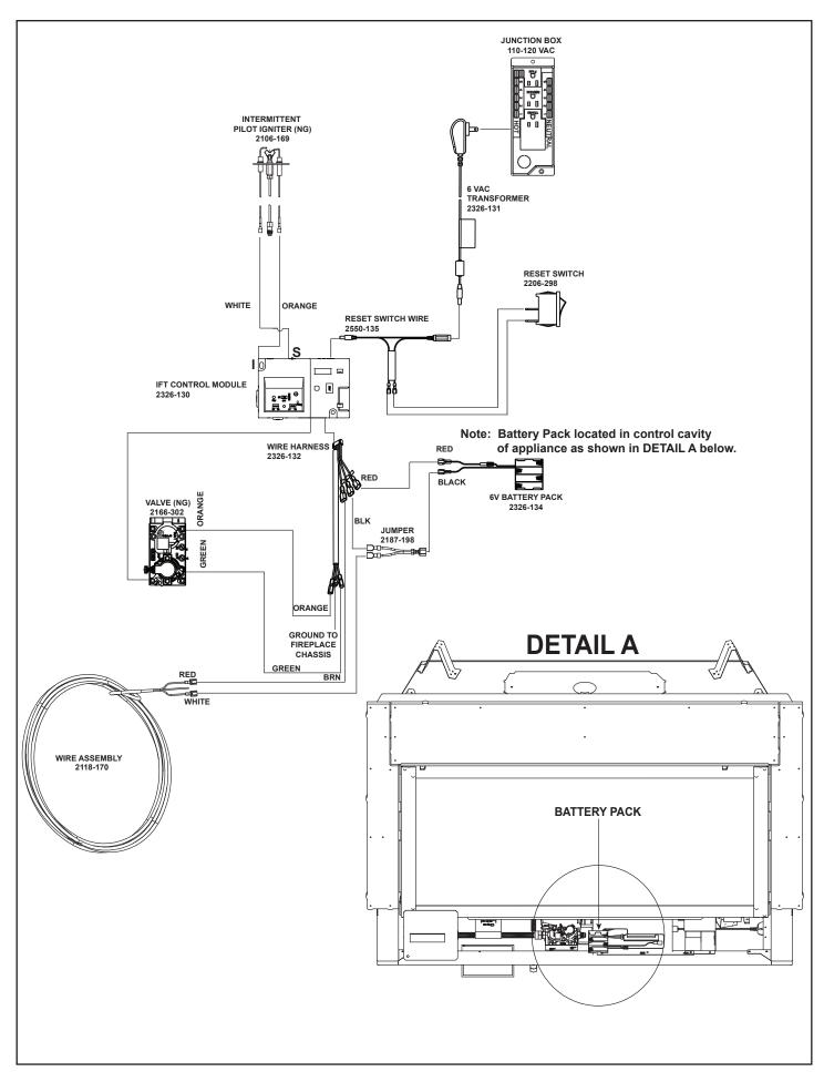
Figure 8.5 Intellifire Touch Wiring Diagram - Standard
