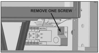
Figure 8.3 Junction Box Detail - JADE32IN-B
