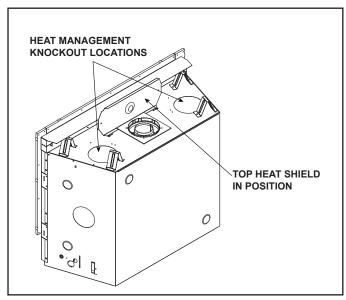
Figure 6.2 JADE42IN-B / JADE42IL-B - Top Heat Shield in Position
