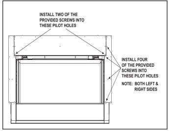
Figure 6.8 Installation of the Side Non-Combustible Components
