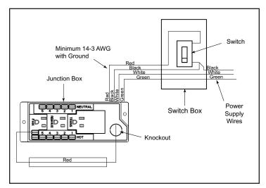
Figure 8.8 Junction Box Wired to Wall Switch
