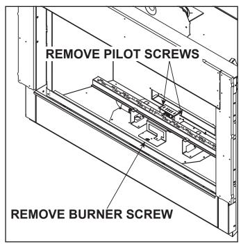
Figure 9.2 Burner Removal
