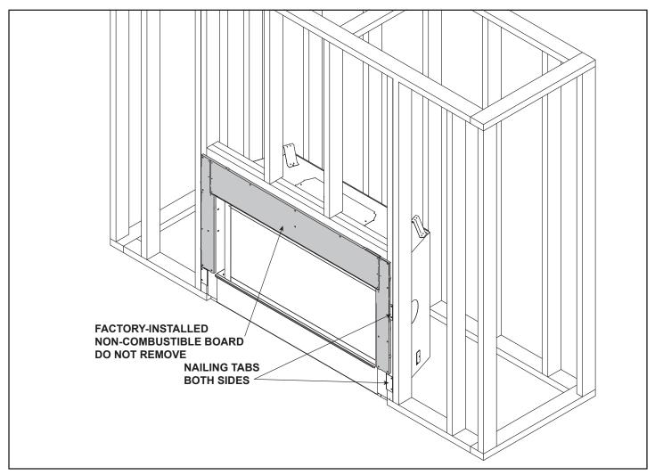
Figure 6.6 Proper Positioning, Leveling And Securing Of Appliance
