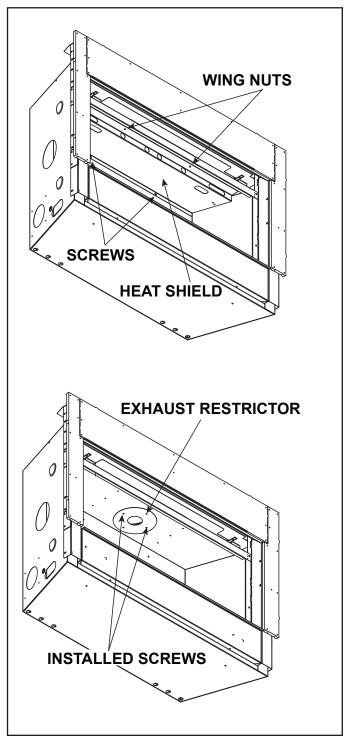
Figure 4.17 Installing Restrictor
