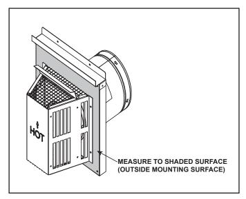
Figure 4.8 Measure to Outside Mounting Surface
