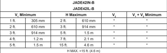
$V_1 + V_2 + H MAX. = 40 \text{ ft. (12.2 m)}$
