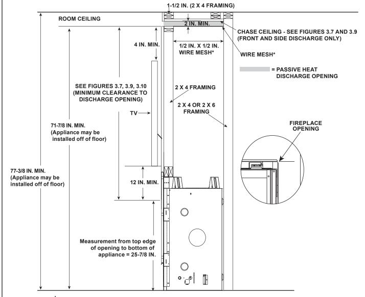
Wire mesh required for front discharge or open top discharge passive heat installations with discharge opening of three inches or greater.
