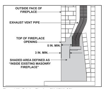
Figure 4.22 Existing Fireplace DV-46DVA-GCL Clearance Requirements
