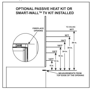
Figure 2.2 Good Faith Wall Surface Temperatures Above Appliance with Passive Heat Kit Installed
