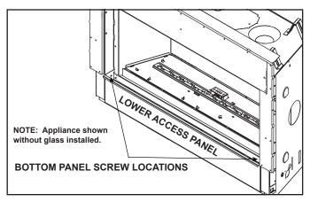
Figure 8.1 Remove Lower Access Panel
