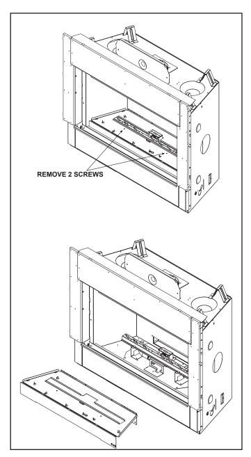
Figure 9.1 Basepan Removal - JADE42IN-B Shown
