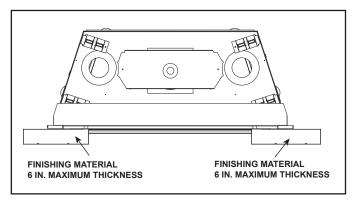
Figure 10.11 Maximum Finish Material Thickness - CFTF Decorative Barrier Front
