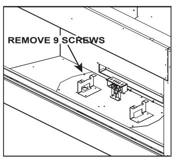
Figure 9.3 Remove Valve Plate
