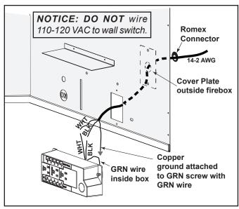
Figure 8.4 Junction Box Detail (Generic Model Shown)
