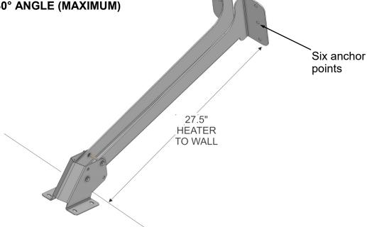
HEATER BRACKET FASTENS TO MOUNTING ARM WITH 2 EACH NUTS & BOLTS SUPPLIED
