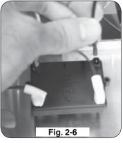
Connect wire to the ignitor module
