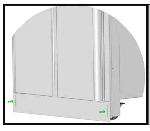
Once you've finished installing the controller, lock the front casters, and push them inward, so that they don't protrude from the font of the grill. Using the other two stainless screws included in the kit, fasten the bottom bracket to cover the casters. The elongated slots on this bracket are to allow for the up/down adjustment of the side brackets.
