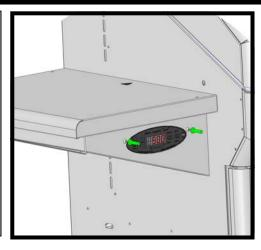
2 Loosen Bolts Using a 3/8" or adjustable wrench, loosen the five bolts that hold the side shelf to the grill. Repeat this on the other side of the grill. You do not need to fully remove the bolts.
