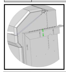
The side brackets mount the same way that the side shelves do— through keyhole slots, sandwiched between the washer and the bolt-head. The elongated keyholes allow the bracket to be adjusted to your countertop height. The Pro can be adjusted from 34.5" to 36". The Elite can be adjusted from 35.5" 37".
