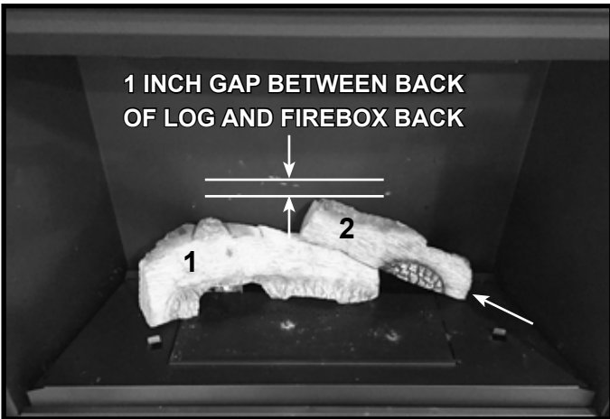
Figure 5. Install Right Rear Base Log
