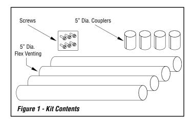
CAUTION: Flex pipe should be stretched out from its compressed state before installation. DO NOT over stretch the Flex. Make sure the flex pipe is slightly loose (but not sagging) when installed to allow for expansion and contraction. Flex pipe must not come in contact with combustible materials. Excessively loose flex could contact combustible materials and cause a fire hazard.
