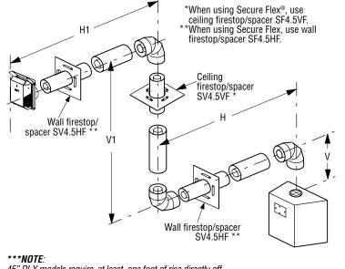
45" DLX models require, at least, one foot of rise directly off unit before connection of elbow.
