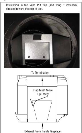
Figure 14B - Vent restrictor installation, Rear vent
