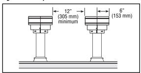
Terminate single vent caps relative to building components according to *Table 6*.
