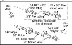
These fireplaces are equipped with a gas flex line for use (where permitted) in connecting the unit to the gas line. A gas flex line is provided to aid in attaching the direct-vent fireplace to the gas supply. The gas flex line can only be used where local codes permit. The flex line is rated for both natural and propane gas. A manual shut off valve is also provided with the flex line.
