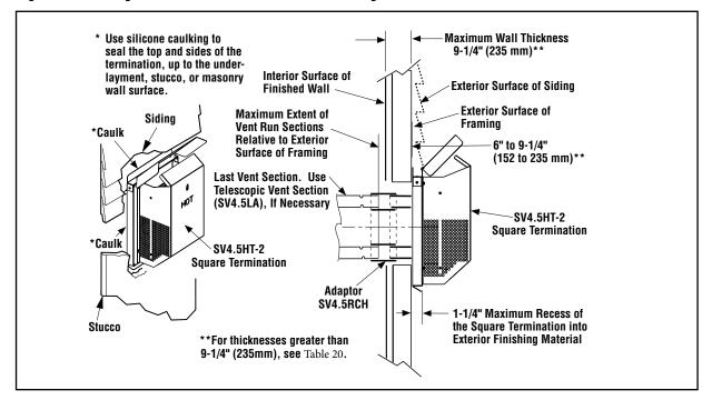
Table 20 - Venting Components Required for Various Exterior Wall Thicknesses, when using Typical Termination Kits
