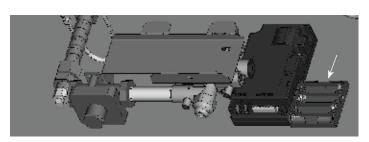
Figure 38B- Battery Holder (in control compartment)
