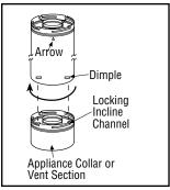
Figure 15B - Connected vent components
