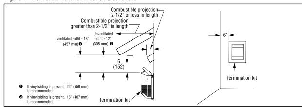
Table 7 - Horizontal vent termination clearances for buildings with combustible and noncumbustible exteriors
