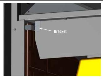
Figure 39C - Brackets Installed
