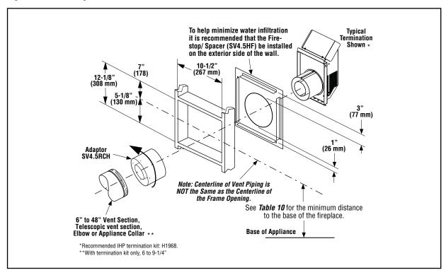
**NOTE:** To help minimize water infiltration install the firestop/spacer (SV4.5HF) on the exterior side of the wall. The firestop may be caulked with mill base caulk (such as 10K81) or high-temperature silicone.
