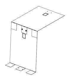
STEP 4. Attach the two (2) shields to the fireplace.
