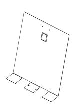
**STEP 3**. Attach the two (2) shields, as shown, with screws.
