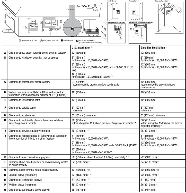
In accordance with the current CAN/CGA-B149.1 National Gas And Propane Installation Code
