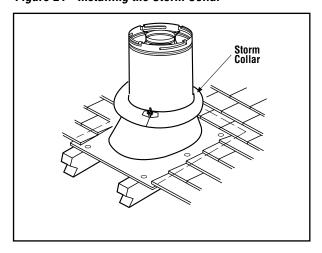
Figure 22 - Installing the Vertical Termination
