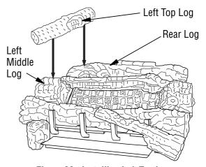
Figure 32 - Installing Left Top Log
