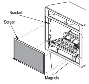
Figure 38 - Installing Fireplace Screen
