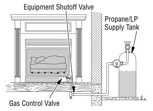
Figure 23 - Checking Gas Joints for Propane/ LP Gas
