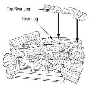
Figure 34 - Installing Top Rear Log
