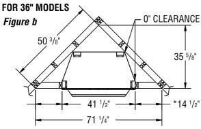
\* THESE DIMENSIONS ALLOW FOR MINIMUM CLEARANCES TO A 45° PROJECTED SIDE WALL
