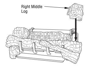
Figure 29 - Installing Right Middle Log
