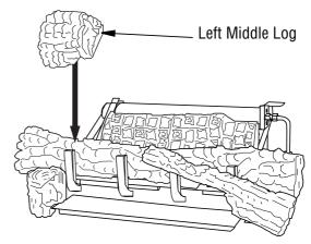
Figure 28 - Installing Left Middle Log
