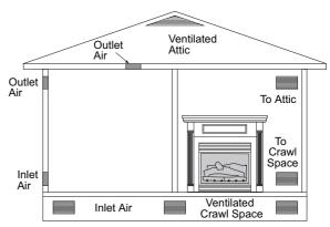
Figure 4 - Ventilation Air from Outdoors
