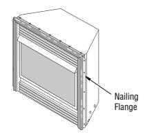
Figure 11 - Location of Nailing Flange
