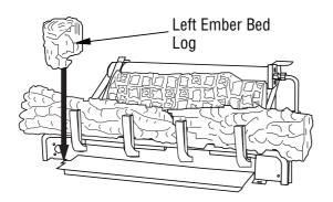
Figure 26 - Installing Left Ember Bed Log
