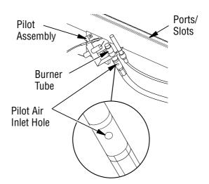
Figure 46 - Pilot Inlet Air Hole
