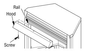
Figure 5 - Installing Hood
