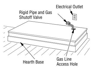
Figure 9 - Placing Hearth Base Accessory
