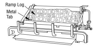
Figure 24 - Installing Fiber Ramp Log
