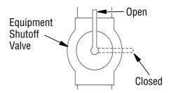
Figure 21 - Equipment Shutoff Valve
