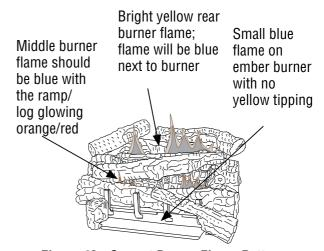
Figure 43 - Correct Burner Flame Pattern
