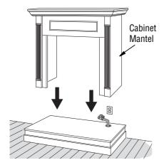
Figure 10 - Installing Cabinet Mantel
