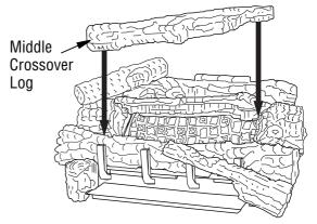
Figure 33 - Installing Middle Crossover Log
