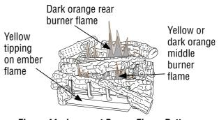
Figure 44 - Incorrect Burner Flame Pattern
