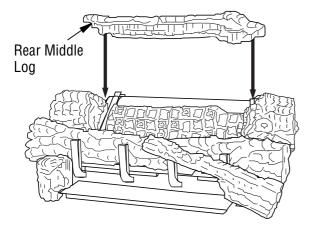
Figure 30 - Installing Rear Middle Log
