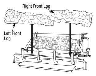
Figure 25 - Installing Left/Right Front Logs
