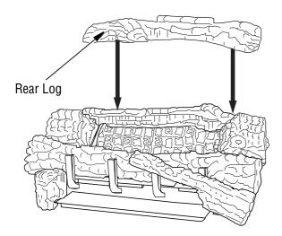
Figure 31 - Installing Rear Log
