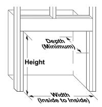
Figure 13 - Rough Opening for Installing in Wall
