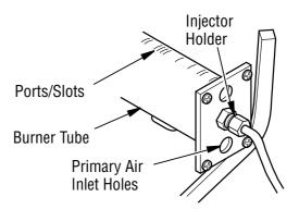
Figure 50 - Injector Holder On Outlet Burner Tube
