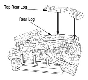
Figure 38 - Installing Top Rear Log
