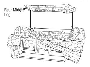
Figure 34 - Installing Rear Middle Log
