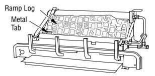
Figure 28 - Installing Fiber Ramp Log
