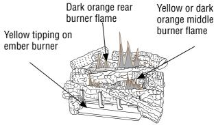
Figure 49 - Incorrect Burner Flame Pattern
