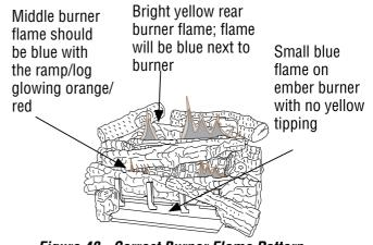
Figure 48 - Correct Burner Flame Pattern
