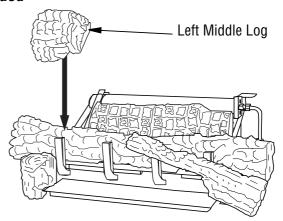
Figure 32 - Installing Left Middle Log
