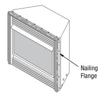
Figure 11 - Location of Nailing Flange
