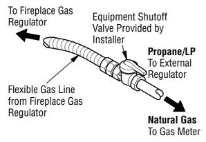
Figure 20 - Attaching Flexible Gas Lines Together
