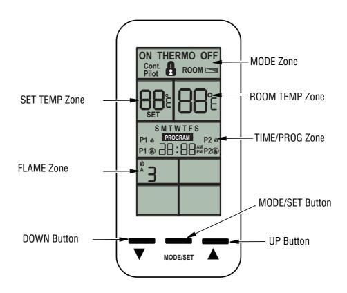
Figure 43 - Touch-Screen LCD and Button Layout
