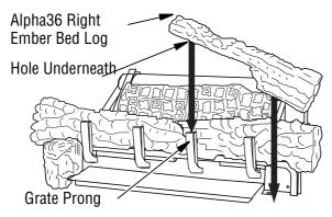
Figure 31 - Installing Right Ember Bed Log
