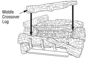
Figure 37 - Installing Middle Crossover Log
