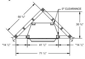
\* THESE DIMENSIONS ALLOW FOR MINIMUM CLEARANCES TO A 45° PROJECTED SIDE WALL
