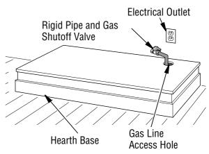
Figure 9 - Placing Hearth Base Accessory
