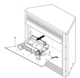
Figure 19 - Removing Log Base Assembly From Fireplace
