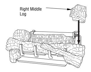
Figure 33 - Installing Right Middle Log
