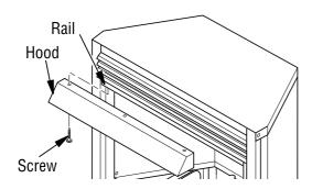
Figure 5 - Installing Hood
