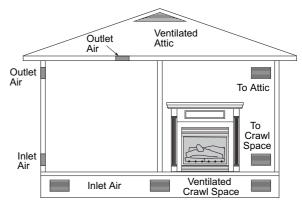
Figure 4 - Ventilation Air from Outdoors
