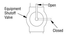
Figure 21 - Equipment Shutoff Valve
