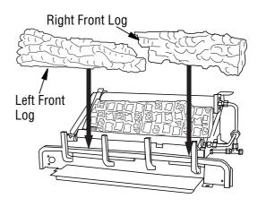
Figure 29 - Installing Left/Right Front Logs
