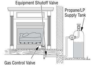
Figure 23 - Checking Gas Joints for Propane/ LP Gas
