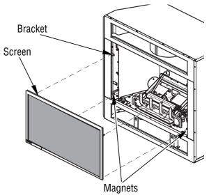
Figure 42 - Installing Fireplace Screen
