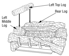
Figure 36 - Installing Left Top Log
