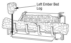
Figure 30 - Installing Left Ember Bed Log
