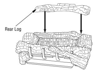
Figure 35 - Installing Rear Log
