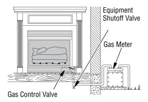
Figure 22 - Checking Gas Joints for Natural Gas
