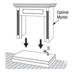
Figure 10 - Installing Cabinet Mantel
