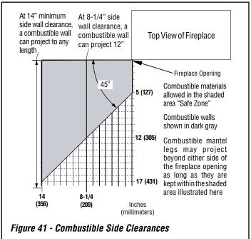
**NOTE:** NEVER install combustible material (wall finish, surround, trim, etc.) on, in front of, or overlapping any part of the fireplace front face.
