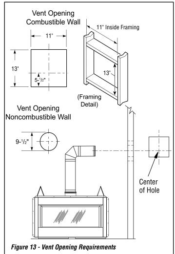
5. Noncombustible Exterior Wall: Position horizontal vent cap in center of the 9-1/2" round hole and attach to exterior wall with four fasteners. Before attaching vent cap to exterior wall, run a bead of non-hardening mastic (pliable sealant) around outside edges to make a seal between it and outside wall.
