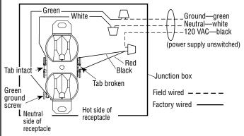
Figure 37A - Junction Box Wiring , 120 V, 60 hz, 1 phase
