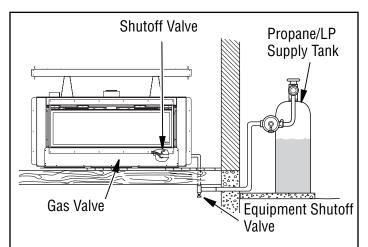
Figure 30 - Checking Gas Joints for Propane/LP Gas Fireplace
