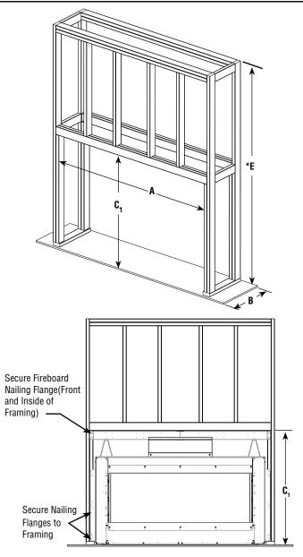
Figure 4 - Framing Flush Wall (Standard Installation)
