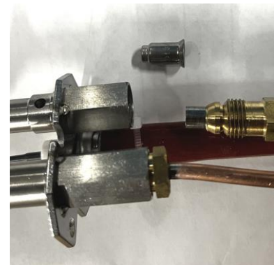
Figure 9.3 – Cleaning pilot orifice
