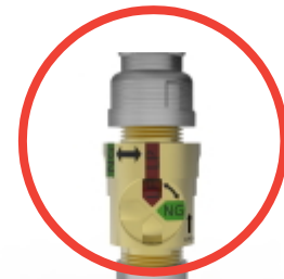
Figure 9.1 – Locating orifice for cleaning
