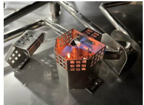
Figure 9.2 – Pilot flame coverage of thermocouple.
