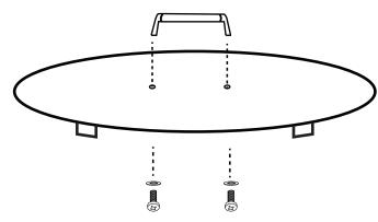
Fig. 1 Installing handle, screws, washers on lid.
