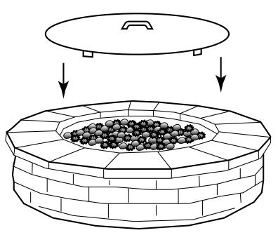
Fig. 2 Installing lid on fire pit closure.
