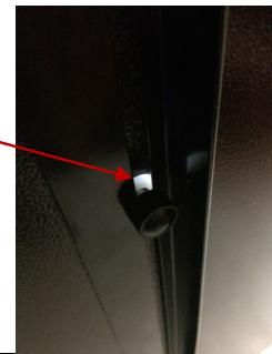
24. To extend the retractable tool holder slide the tool holder upward until the plastic head screws can be steered into the “hooks” on the left side of the slot in the tool holder.
