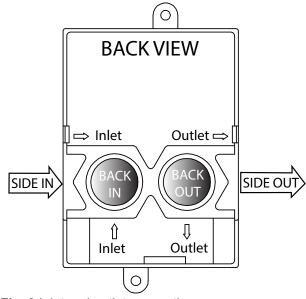
Fig. 2 Inlet and outlet connections.
