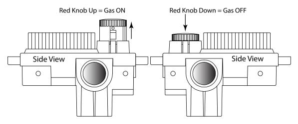
Fig. 5 E-Stop Gas Timer red knob positions
