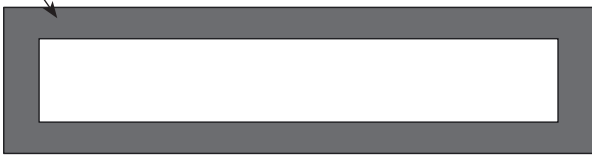
Figure 1 - Evenly Apply Adhesive to Back of Surround Face (Back View Shown)
