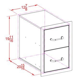
PERSPECTIVE VIEW WITH INSTALLATION CUT OUT DIMENSIONS
