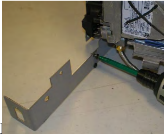
1 Remove On/Off Switch and original mount bracket.
