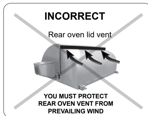
Fig. 17-4 Airflow direction - INCORRECT
