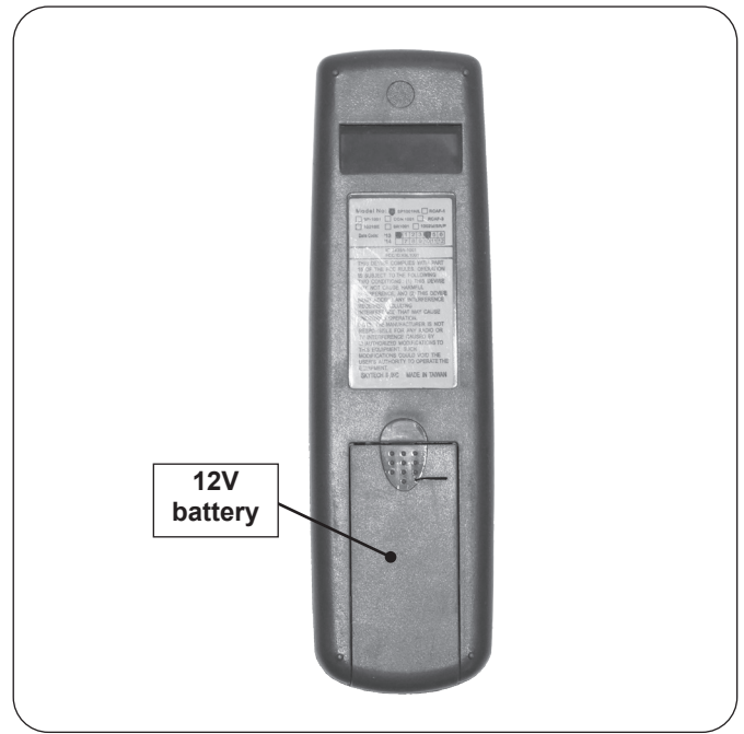
Fig. 15-1 Install transmitter battery
