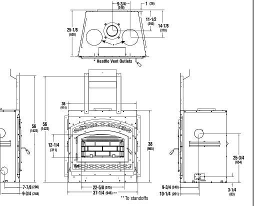
Figure 11 - Framing Dimensions
