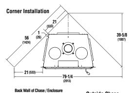
\* Zero Clearance from Back Spacer to Wall
