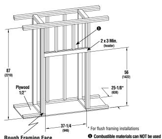
Rough Framing Face (dimension includes finish material inside framing, if any)
