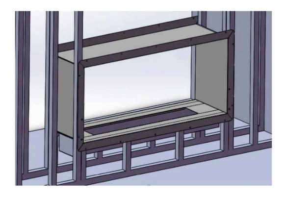
5. Install a stud horizontally on top of the firebox to be able to continue with the wall 6. Screw the top of horizontal stud directly to the Firebox brackets (use 0.5 inch metal zips)
