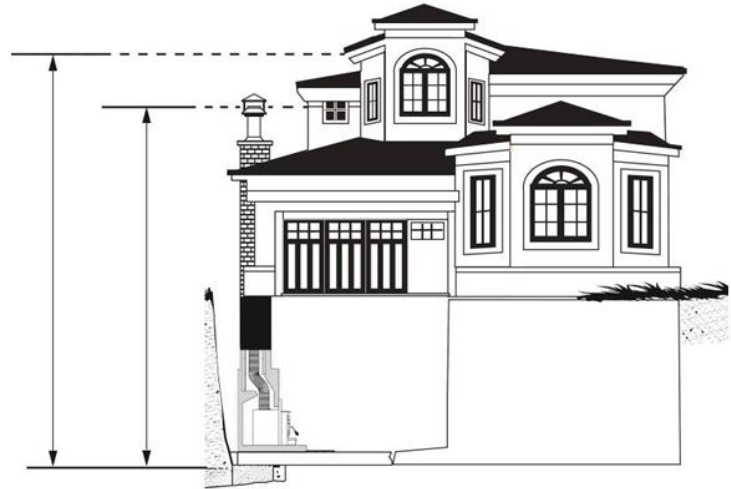
Figure 29: Chimney location in the house
