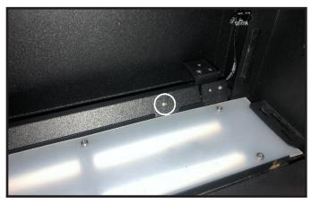
Figure 18 Light Shield Removal
