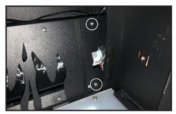
Figure 14 Side Panel Removal
