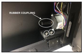
Figure 17 Rubber Coupling and Motor Removal
