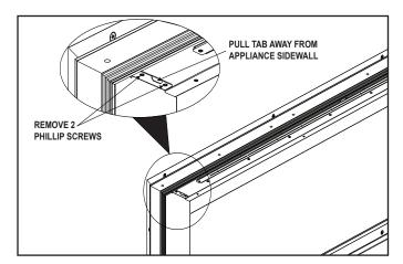
Figure 6 Side Panel Removal
