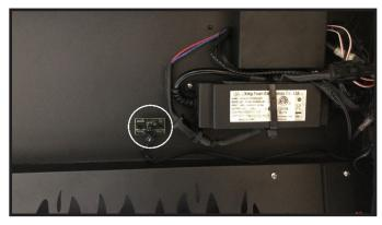
Figure 11 Receiver Board Removal
