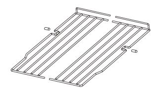
When removing the shelf from the inner rails, move to the position where the notches in the shelf are exactly aligned with plastic posts and lift the shelf. In order to replace the shelf, repeat this procedure in reverse.
