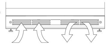
NOTE: It is recommended that you do not install the appliance near an oven, radiator or other heating source. Direct sunlight may affect the acrylic costing and heat sources may increase electrical consumption. Don't install in a location where the temperature will fall below 44°F (7°C). For best performance, do not install the appliance behind a cabinet door or block the base grille.
