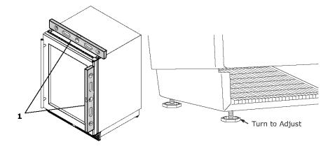
For free standing, 5 inches (127mm) of space between the back and sides of the unit are suggested, which allows for proper air circulation to cool the compressor and condenser. Even built-in installations require a minimum of 1/4" (6.35mm) space on each side and at the top. TAKE CARE THAT THE AIR VENT AT THE FRONT OF THE APPLIANCE IS NEVER COVERED OR BLOCKED IN ANY WAY.
