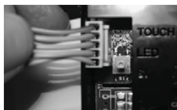
Figure 20 - Connecting end of Touch Pad Cable
