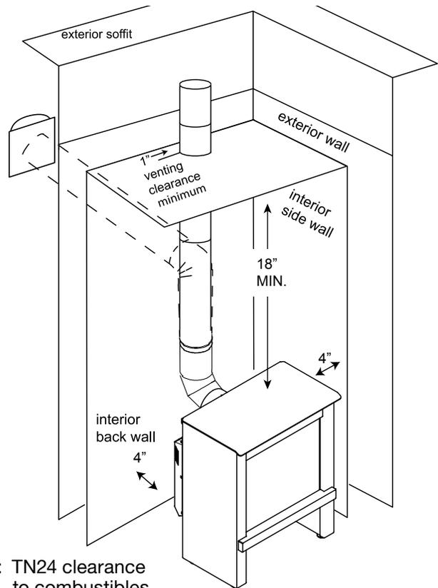
Figure 23: TN24 clearance to combustibles.
