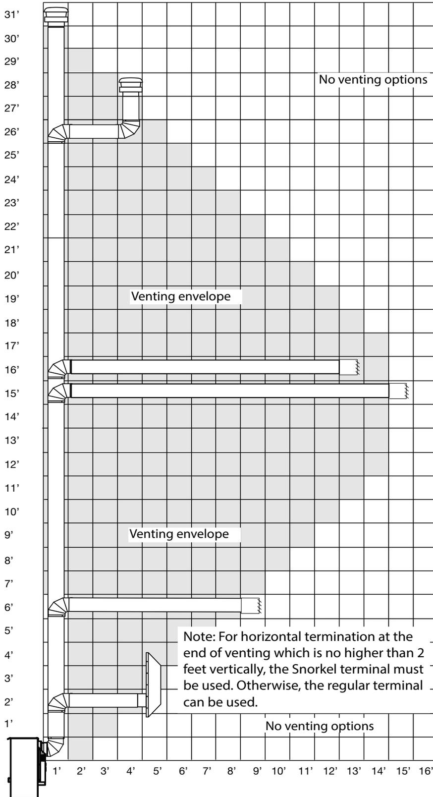
Note: The vent must not exceed a total length of 30 feet. Any combination of rise and run may be used but must be constrained to the boundaries of this chart. A Maximum of three (3) 90° elbows may be used. Only one (1) 90° elbow or combination of other elbows equaling 90° can be used without reducing horizontal run. For each additional 90° elbow, or an equal combination of elbows, reduce horizontal vent run by 2 feet. Ensure vent pipe is properly supported.
