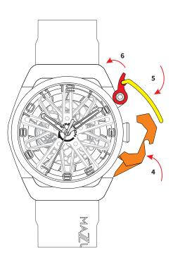
4 CLOSE THE PROTECTIVE ARM 5 CLOSE THE WIRE CLASP 6 LOCK THE HOOK
