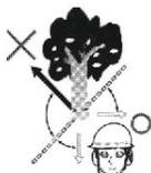
5. Never start cutting until you have a clear work area, secure footing, and a planned retreat path from the falling tree.
