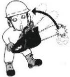
18. Do not operate the chain saw in a tree unless specially trained to do so.
