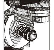
E. Adjust the stop screw (13) to control the amount of cutter to be filed.
