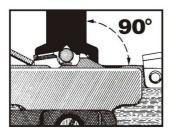
C. Insert file into the cutter, making sure file assembly is positioned at 90° to the T-bars (5).
