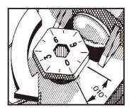
F. Rotata adjusting screw (12) counter-clockwise to the recommended depth gauge setting (see chain chart or chain manufacturer's instructions for recommended setting).
