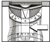
B. Set both filing angles to 0° so that the file is 90° to the guide bar.
