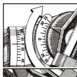
B. To sharpen cutters on the opposite side of the chain, unlock swivel knob (10) and rotate swivel guide (2) to the similar setting on the opposite side.
