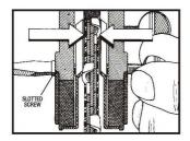
E. Secure T-bars (5), by using thumb screw (6) and opposing slotted screw, to center the chain and stabilize cutter for sharpening.
