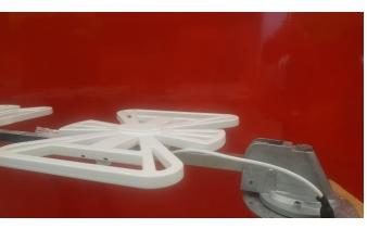
Now the Mast has been retro-fitted to the Antennatek Base, test mast operation with the crank handle to bring it to an upright position. Keep it upright to make routing the Coax Cable much easier.
