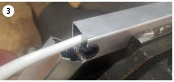
Slide Coax Cable from access hole so it sits out, and remove.
