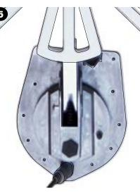
Insert the pin through the leveling bracket and the elevating gear. Push the e-clip over the end of the pin.
