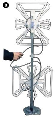
Continue to thread the coax in an S-curve. Thread the coax over and then under the boom.
