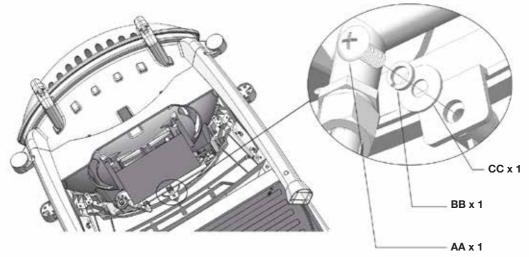
Position the heat shield tabs as shown into the slot on the fat tray support.
