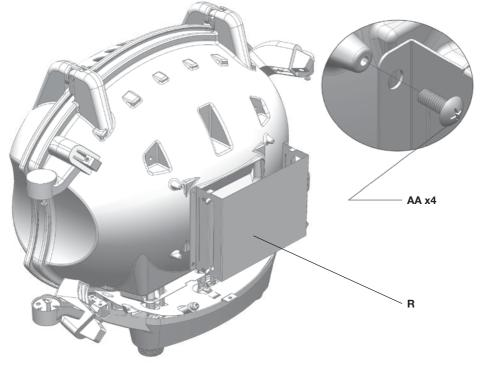
Locate the barbecue body as shown and secure with the four fasteners. Plug the holes as shown.
