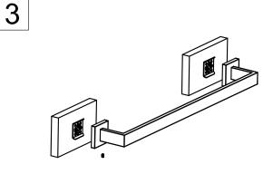
Slide body assembly onto mounting bracket.
