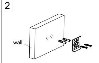
Install mounting bracket to the wall with screws(supplied) and anchors(if applicable).
