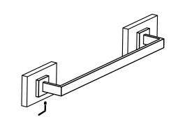
Tighten set screw with allen key (supplied).
