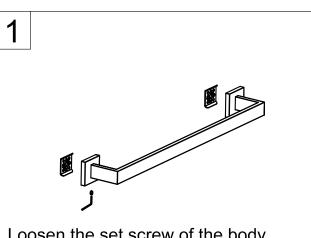
Loosen the set screw of the body assembly, pull out the mounting bracket.
