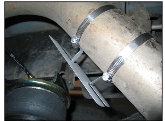
Passenger side front. Installation of E-brake line.
