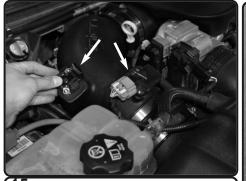
**15.** Place both MAF sensors onto their appropriate location and then screw them down with the supplied M4 bolts. Reconnect the MAF sensor harnesses
