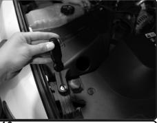
**16.** Reuse the factory 8mm bolt and secure the Injen air box bracket to the passenger side headlight bracket.
