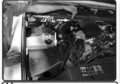
**14.** First slide the big end of the intake pipe into the 5.0" hump hose on the air box plenum. Then slip the smaller end into the 4.25"-4.50" step hose on the turbo inlet. Once intake is adjusted, tighten all clamps.
