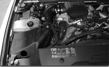
Congratulations! You have just completed the installation of this intake system. Periodically, check the alignment of the intake, normal wear and tear can cause nuts and bolts to come loose. <u>Note: Check clearance and</u> <u>adjust if needed! Failure to check the</u> <u>alignment and adjust the intake can</u> <u>cause damage that will void the warranty.</u> <u>Injen Technology is not responsible for</u> <u>any damages caused by/from improper</u> installation.
