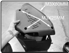
**8.** Place the three M6X25mm bolts and one M6X80mm into the plenum illustrated by the photo. Your Injen air box assembly is now complete.
