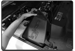
**11.** Lower the Injen air box into the engine bay. Make sure the pegs under the Injen air box goes into the factory air box grommets on the air box tray from figure 10
