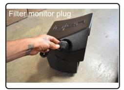
**5.** Place the Filter Minder plug into the hole in the Injen air box
