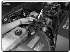
Remove the factory torx screws from the MAF sensor and then remove the MAF sensor from the factoryu air box assembly.
