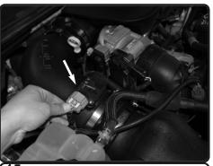
**15.** Place the MAF sensor onto the intake tube and then secure it with the supplied M4 bolts. Reconnect the MAF sensor harnesse
