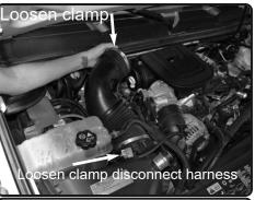
Disconnect the MAF sensor harness.Loosen the clamp on the intake duct and then remove entire air duct
