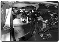
**14.** First slide the big end of the intake pipe into the 5.0" hump hose on the air box plenum. Then slip the smaller end into the 4.25"-4.50" step hose on the turbo inlet. Once intake is adjusted, tighten all clamps.
