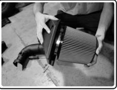
**7.** Place the filter onto the the Injen intake plenum and then secure the clamp.
