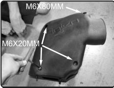
**8.** Place the three M6X20mm bolts and one M6X80mm into the plenum illustrated by the photo
