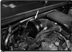
**9.** Place the 4.25X2.75" Straight hose and two #72 clamps on to the turbo inlet. Secure the clamp on the turbo inlet only for now
