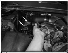
**16.** Place the MAF sensor into the Injen tube. Secure the MAF sensor to the tube with two M4 button head bolts. Reconnect the MAF sensor harness
