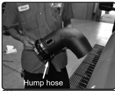
**13.** Place the 5.00" hump hose and two #80 clamps onto the big end of the Injen intake tube
