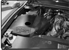
**12.** Drop the Injen air box onto the grommets from figure 11. Make sure the two mounting nipples underneath the Injen air box goes directly into the grommets.
