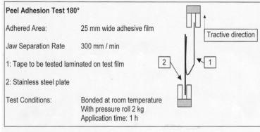
Test Result At 20 mins = 26 N/25 mm
