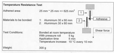
Test Result =  $-40 \, {}^{\circ}\text{C} / + 80 \, {}^{\circ}\text{C}$
