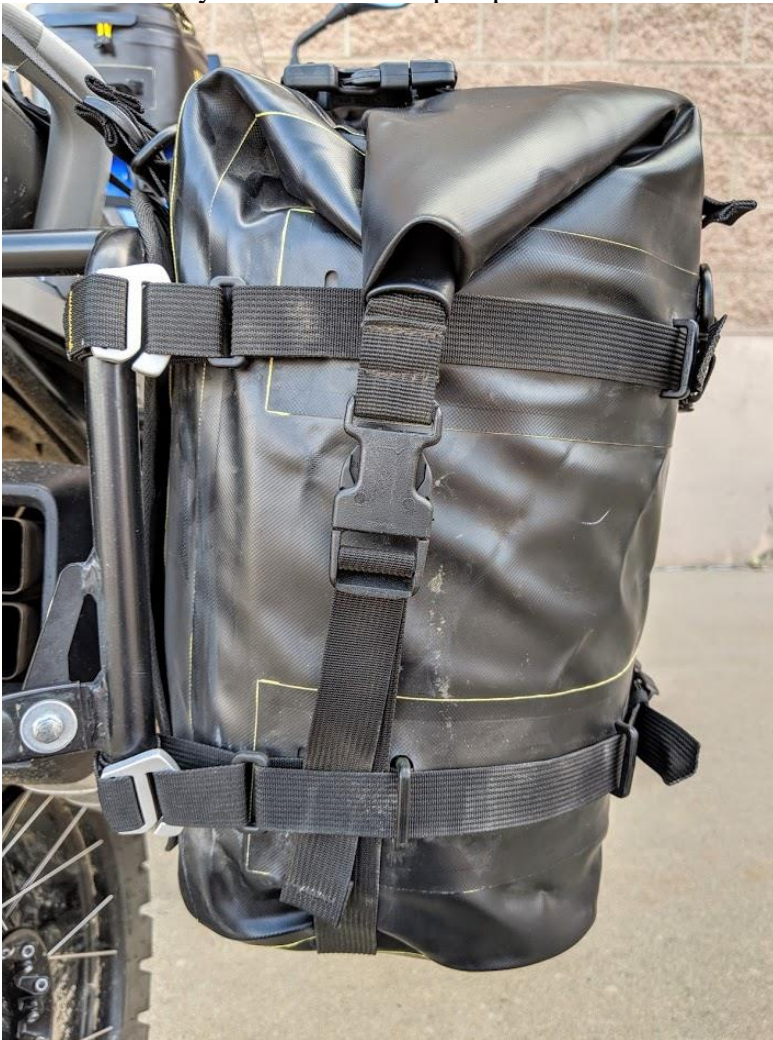
FIG12 Correctly Fastened G-Hoop Top and Bottom
