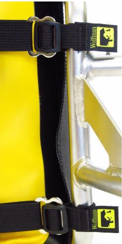
8- Tighten the 1" Side mounting straps threaded through each cam buckle on front of each bag. FIG.10 Tighten straps to secure and compress bag to the rack (pull side mounting straps away from the cam buckles in the direction of the arrows).
