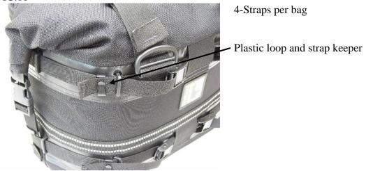
10- Tighten the 2" wide seat straps by pulling the webbing away from the 2" buckles. You can pull both ends to tighten the webbing. FIG.12
