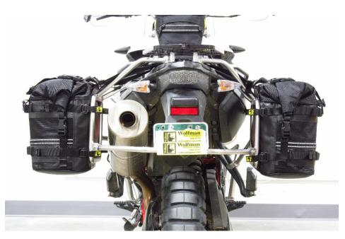
FIG.5 (This is a rear view of a properly adjusted set of saddle bags)
