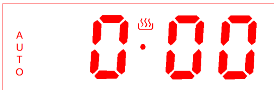
Pic 14 Cooking time setting initial state
