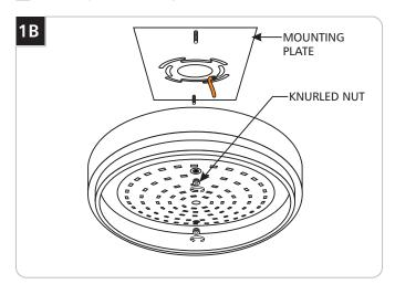
Remove the mounting plate from the fixture base by unscrewing the two knurled nuts.
