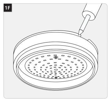
**9 For wet location installation,** caulk around the fixture base with waterproof construction sealant.
