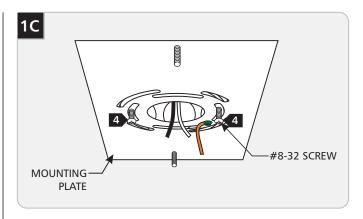
4 Secure the mounting plate to the electrical box with 2 #8-32 screws.
