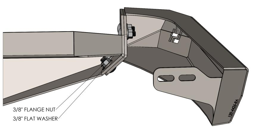
NOW THAT THE CARRIAGE BOLTS AND SIDE WING ARE IN PLACE, SECURE USING THE SUPPLIED 3/8" FLAT WASHER AND 3/8" FLANGE NUT RESPECTIVELY. LOOSELY TIGHTEN AND REPEAT ON DRIVER/ PASSENGER SIDE WING. FLIP BUMPER OVER TO ENSURE BOTH ARE FLAT, THEN TORQUE ALL (8) NUTS TO 45 FT-LBS.
