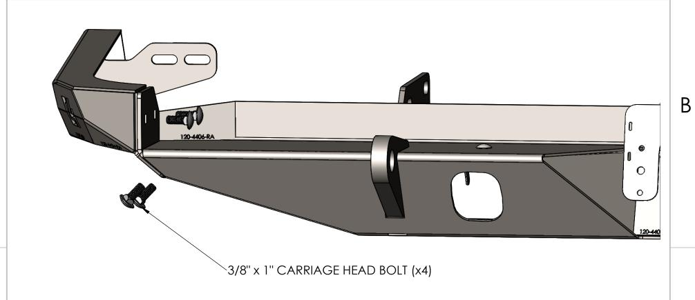
INSERT THE (4) 3/8" x 1" CARRIAGE HEAD BOLTS AS SHOWN INTO SIDE WING
