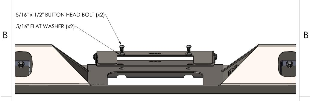
PLEASE REFER TO THE LICENSE PLATE MOUNT BRACKET INSTRUCTIONS TO SHOW HOW TO ASSEMBLE THE FLIP UP BRACKET. ONCE FLIP UP BRACKET IS ASSEMBLED, MOUNT IT TO THE BUMPER AS SHOWN USING THE SUPPLIED 5/16"x1/2" BUTTON HEAD BOLTS AND 1/4" FLAT WASHERS, PASSING THROUGH THE FLIP UP BRACKET AND MOUNTING TO THE WELDED NUTS IN THE BUMPER.
