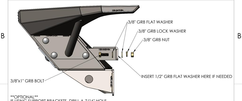
IF USING SUPPORT BRACKETS, DRILL A 7/16" HOLE IN BODY MOUNT, SECURE BRACKET TO BODY MOUNT USING SUPPLIED 3/8" x 1" GRADE 8 BOLT, 3/8" FLAT WASHERS, 3/8" GR8 LOCK WASHER, AND 3/8" GR8 NUT RESPECTIVELY. IF THERE SUPPORT BRACKET IS NOT FLUSH WITH BODY MOUNT, USE SUPPLIED 1/2" GR8 FLAT WASHER TO FILL GAP. TORQUE TO 55 FT-LBS. REPEAT PROCESS ON PASSENGER SIDE.
