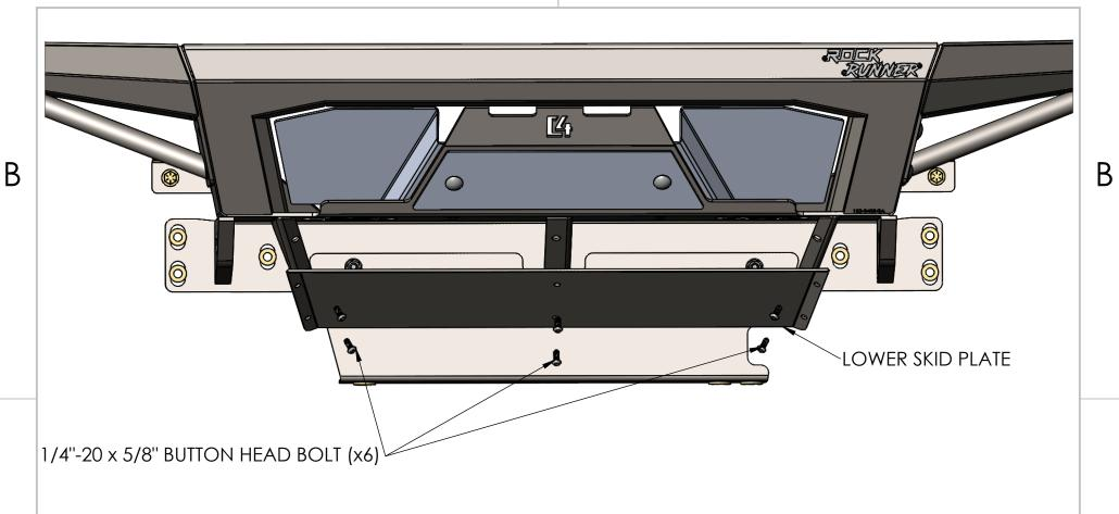
USING THE SUPPLIED 1/4"-20 x 5/8" BUTTON HEAD BOLTS, SECURE THE LOWER SKID PLATE TO THE BUMPER. THERE WILL BE EXISTING NUTS WELDED TO THE BUMPER TO FASTEN BOLTS TO.
