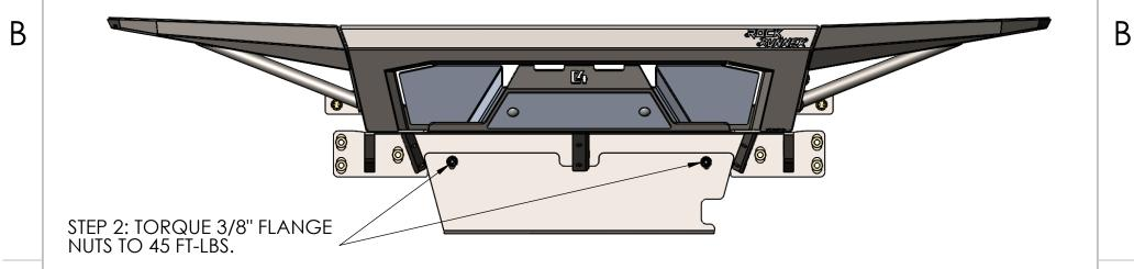
STEP 1: USING EXISTING M10 BOLTS FROM CROSSMEMBER TO SECURE THE CROSSMEMBER FILL PLATE TO THE CROSSMEMBER. TORQUE TO 45 FT-LBS.
