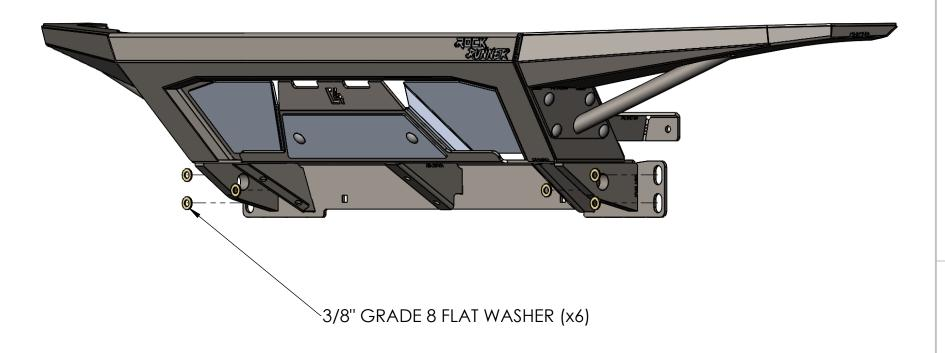
USE SUPPLIED 3/8" GRADE 8 FLAT WASHERS AND EXISTING M8 FLANGE NUTS THAT WAS HOLDING THE CRASH BAR ON TO SECURE THE BUMPER TO THE PICKUP. TORQUE M8 BOLTS TO 55 FT-LBS ON THE FRAME STUDS.
