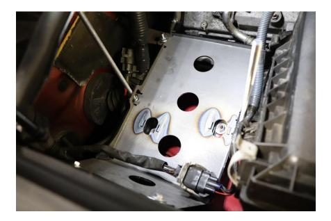
14) Once the tray is secure, the battery can be installed. Set the battery into the tray and position it so that it does not sit on top or pinch the wiring harness with the large square plug.Set the battery hold down clamp down on top of the battery while fitting the all thread studs through the holes at each end of the clamp at the same time.
