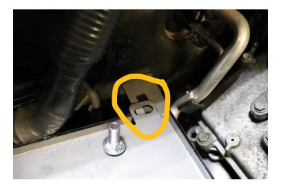
12) Install the 6mm bolts with ¼" washer into the two threaded holes in the side of the engine compartment above the fender.
