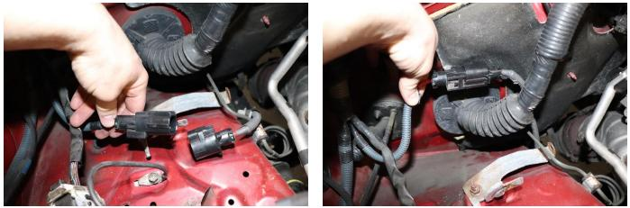
boot coming through the firewall. Secure the wire and connector in place with cable ties.
