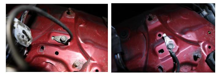
6) Remove the plastic nut from this 6mm stud on the firewall. Loosely install the "L" bracket to the firewall using one ¼" flat washer and the 6mm nut.
