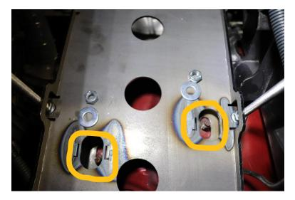
11) Install the 3/8" carriage head bolt through the "L" bracket and the tab at the corner of the tray. Loosely install the 3/8" flange nut onto the bolt.
