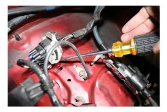
2) Using the flat blade screwdriver, pry open the clip that holds the large round electrical connector to the metal mounting bracket.
