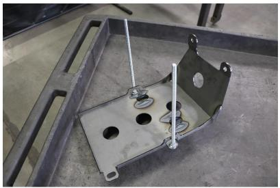
9) Now install the tray into the engine compartment. Tip and rotate the tray to get it into position. Slope the tray so that the vertical portion can go in first and fit under the wiring harness with the large square plug. On some newer models of 4runners the wires with large square plug can be left in position where they are attached to the side of the fender area and the tray will fit around the large connection.
