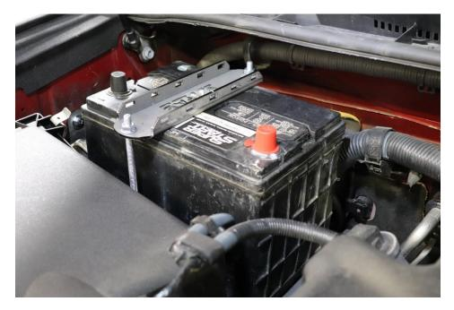
15) Tighten the nuts evenly so the clamp sits flat on the top of the battery and puts even pressure across the top of the battery. Push and pull on the battery to make sure the nuts are tight enough to hold the battery in place under rough driving conditions. Be sure not to tighten the clamp nuts more then what is necessary to hold the battery in place.
