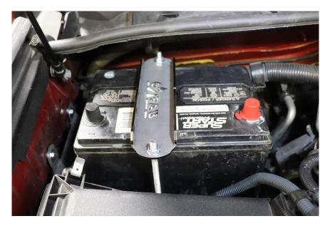
Double check to make sure no wires are pinched or rubbing anywhere on the tray or battery.
