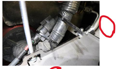
4) Use a 12mm wrench or socket to remove the nut holding the metal bracket to the fender. This bracket will not be needed. This metal bracket is slightly different on newer 4runners but the bracket still needs to be removed and the wire with large connector gets relocated also.
