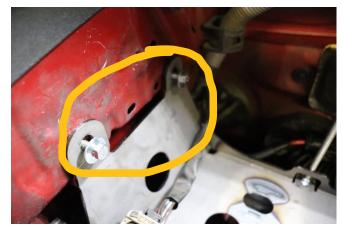
13) Now that all the hardware is loosely installed, adjust the tray so that it sits level. Tighten all hardware to hold the tray in place. Your tray should look like this once everything is tight and in position.
