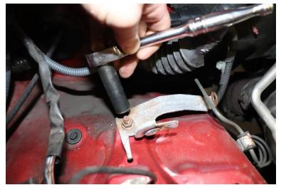
5) Use a 10mm wrench or socket to loosen the bolt holding the ground cable in place. Rotate the cable 90 degrees clockwise so it matches the image. Tighten the bolt to hold the cable in position.
