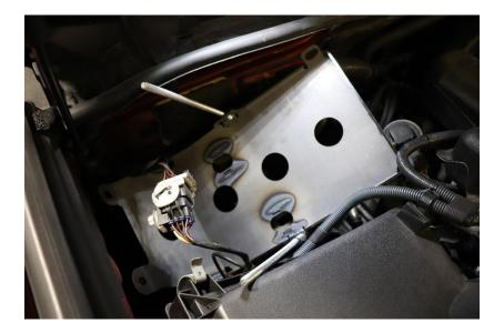
10) Line up the tray with the 8mm studs that are on the fender. Set the tray in place down onto the studs. Loosely install one 5/16" washer and 8mm nut onto each stud.
