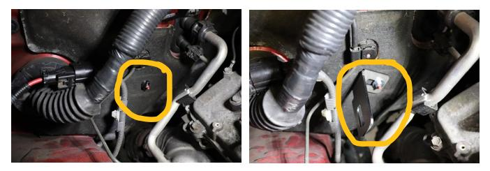
7) Now attach the all thread studs to the battery tray. Thread one 5/16" flange nut onto the stud upside down. Leave about a  $\frac{1}{2}$ " of thread exposed past the nut. Push the stud through the hole on the battery tray. Install another flange nut on the other side and tighten down both nuts.
