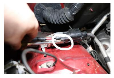
3) Un plug the electrical connection. Route the connection behind the large rubber wiring harness
