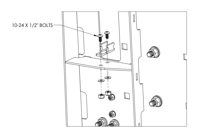
NAME DATE C4 FABRICATION 10/2/18 BEB DRAWN CHECKED **UPPER CATCH** ENG APPR. PROPRIETARY AND CONFIDENTIAL MFG APPR. THE INFORMATION CONTAINED IN THIS DRAWING IS THE SOLE PROPERTY OF Q.A. C4 FABRICATION, LLC. ANY COMMENTS: REPRODUCTION IN PART OR AS A SIZE DWG. NO. REV WHOLE WITHOUT THE WRITTEN PERMISSION OF C4 FABRICATION, LLC IS PROHIBITED. MATERIAL DO NOT SCALE DRAWING WEIGHT: SHEET 27 OF 27
