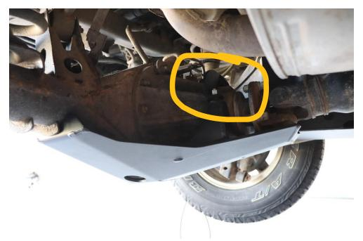
Install the 3/8" split lock washers and 3/8" nuts onto the carriage head bolts and tighten with an open end wrench.
