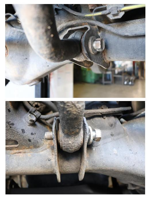
3) Before lifting the skid into position install the two 3/8"x1" carriage head bolts into the diff skid and put some tape over the head of the bolt to hold them into place and stop them from falling out of the hole.
