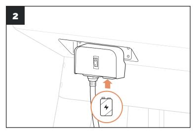
Turn the main power switch on the back of the Flat Top Grill to ON (I). The power switch will illuminate when turned on.
