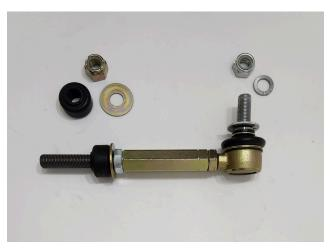
Remove top lock nut, washer, and bushing from the assembly.
