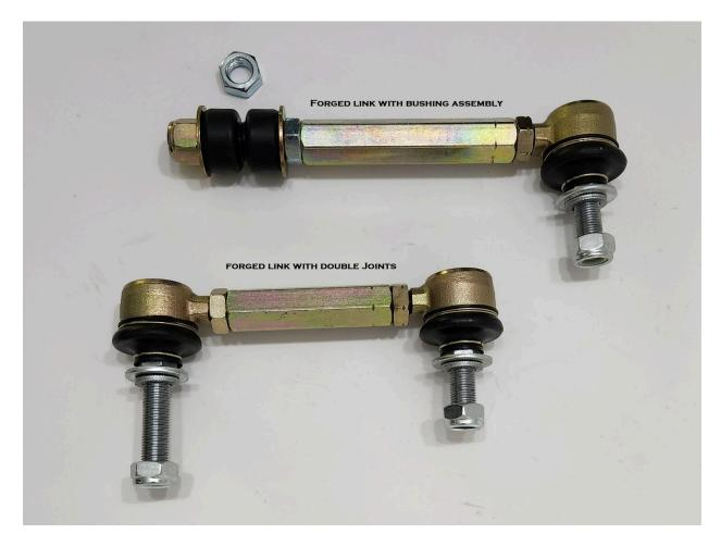
\*All forged joints come pre-assembled and include thread locker.
